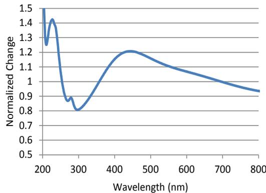
Figure 1. Predicted signal change after endpoint for Type A mask shown at end of etch
