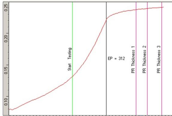
Figure 3. Example endpoint time trace with resist markers illustrating three resist thickness preset levels achieved at successive times.
