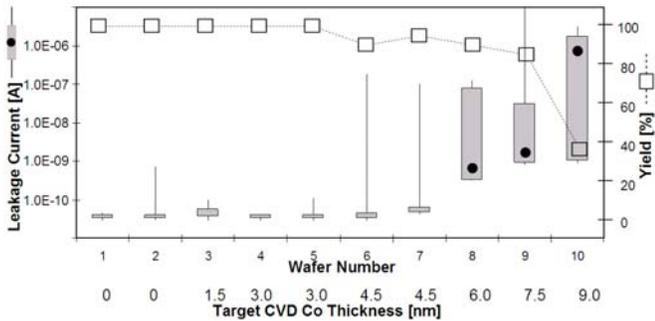
FIG. 1: Leakage measurements from 10 Torr CVD Co process.
