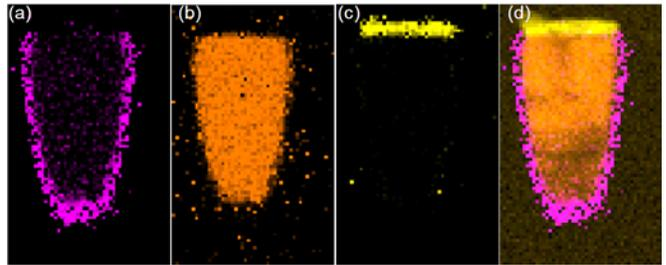
FIG. 6: EDX mapping showing detected (a) Ta at sidewall of the Cu line, (b) Cu, and (c) Co at top surface of the Cu line. (d) Color overlay showing Co covering the Cu surface.
