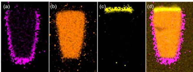
FIG. 4: EDX mapping showing detected (a) Ta at sidewall of the Cu line, (b) Cu, and (c) Co at top surface of the Cu line. (d) Color overlay showing Co covering the Cu surface.
