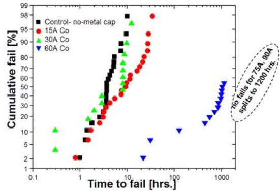
FIG. 8: Distribution of EM fails showing dependency on the deposited Co cap thickness.
