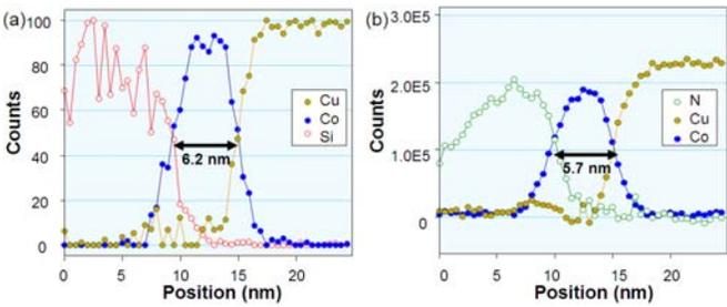
FIG. 3: Co cap thickness measurements from (a) EDX, and (b) EELS. The target thickness is 6nm.
