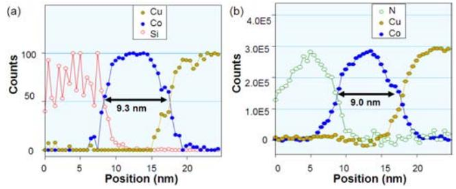
FIG. 5: Co cap thickness measurements from (a) EDX, and (b) EELS. The target thickness is 9nm.
