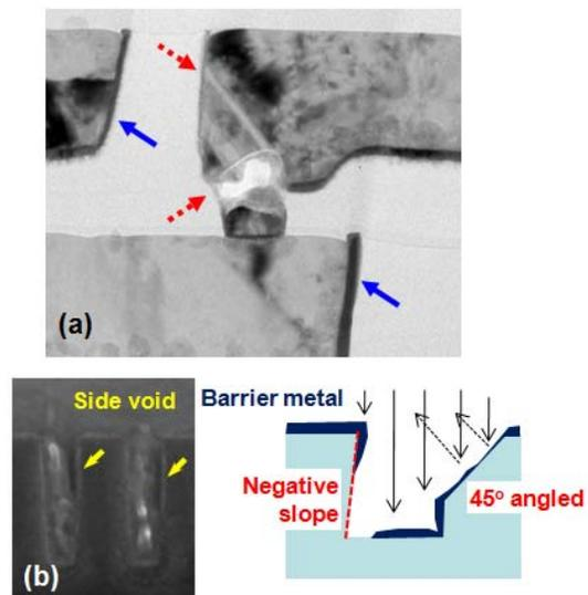
Figure 7. (a) Very thin or discontinuous layers (dashed red arrows) were observed along with the normal coverage (blue solid arrows) in TEM image of PVD TaN\Ta sample after EM test. (b) Vertical SEM image shows the voids during electroplating due to insufficient coverage of barrier metal and seed Cu.
