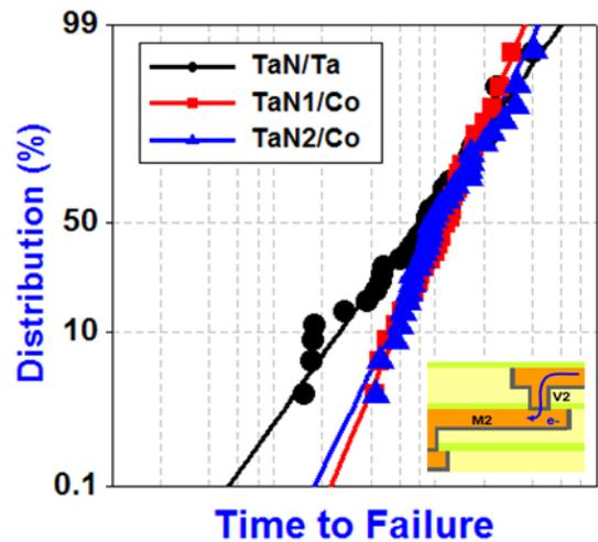
Figure 10. The shift of TTF was not observed in lognormal probability plot of downstream EM like the upstream, but the distribution became stiff by removal of early failures when CVD Co barrier was involved.
