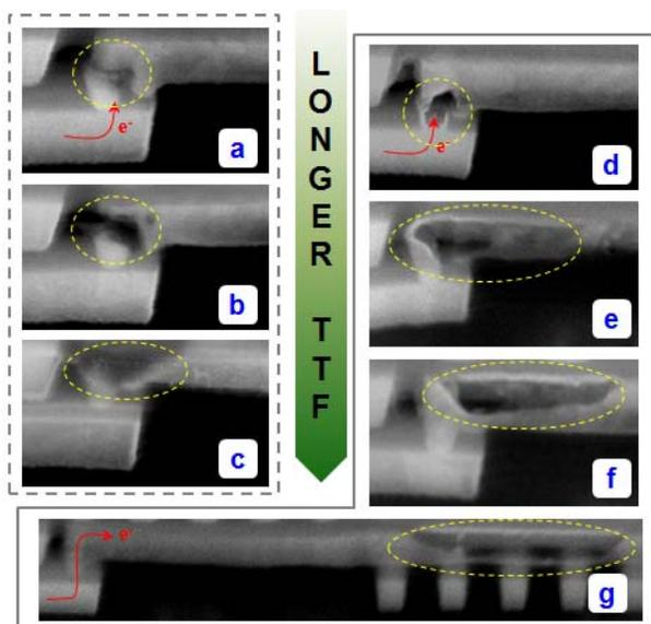
Figure 9. FIB analysis was performed for the samples with the whole range of lifetime that were plotted in Fig. 8; (a)-(c) : TaN/Ta, (d)-(g) : TaN/CVD Co
