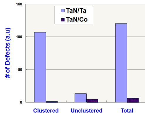
Figure 3. Classified numbers of defects after CMP was significantly decreased by using TaN\Co barrier.
