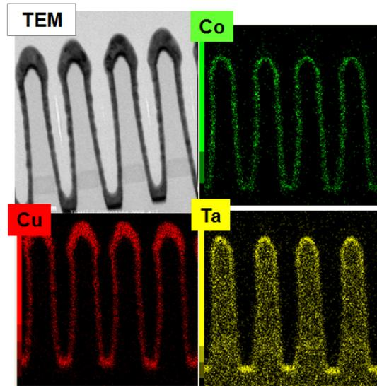
Figure 2. Almost 100% step coverage of CVD Co could be obtained in cross sectional STEM-EDS images of TaN\Co\Cu seed.
