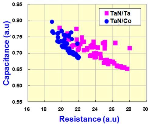
Figure 5. RC value decreased by 10% with the resistance when a TaN\Co stack was applied.
