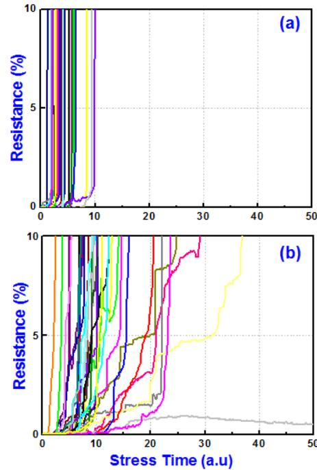
Figure 6. For upstream EM, resistance degradation trends are quite different between two groups ; (a) TaN\Ta, (b) TaN\CVD Co. When CVD Co barrier was adopted, increased MTTFs (median time to failure) and gradual increase in resistance were observed.
