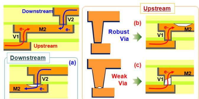
Figure 1. Two types of EM along the current flow was shown.
