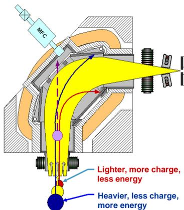
**Figure 3.** Magnet current is set to allow ions of a specific mass, charge, and energy to pass through the resolving aperture, while others are deflected.
