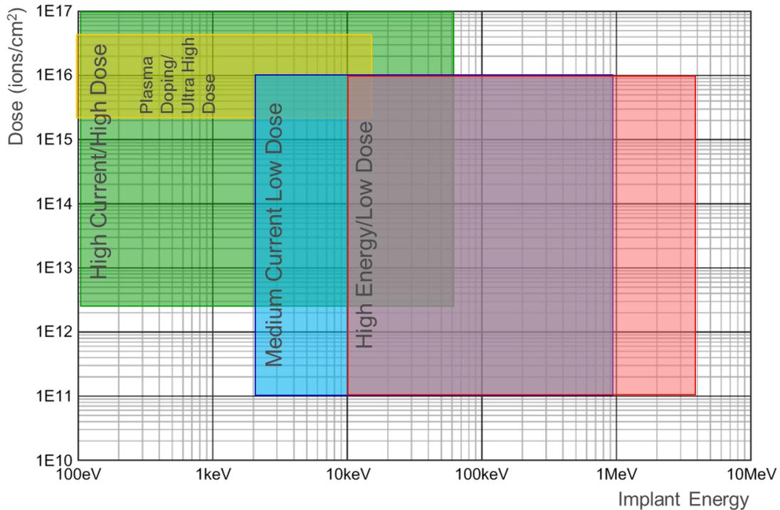
**Figure 5.** The wide range of dose and energy requirements for implant applications exceeds the Capability of one ion beam system; doping three-dimensional devices requires plasma-based technology.
