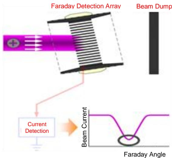
**Figure 4.** Controlling incident beam angle is essential for accurate and repeatable implant.
