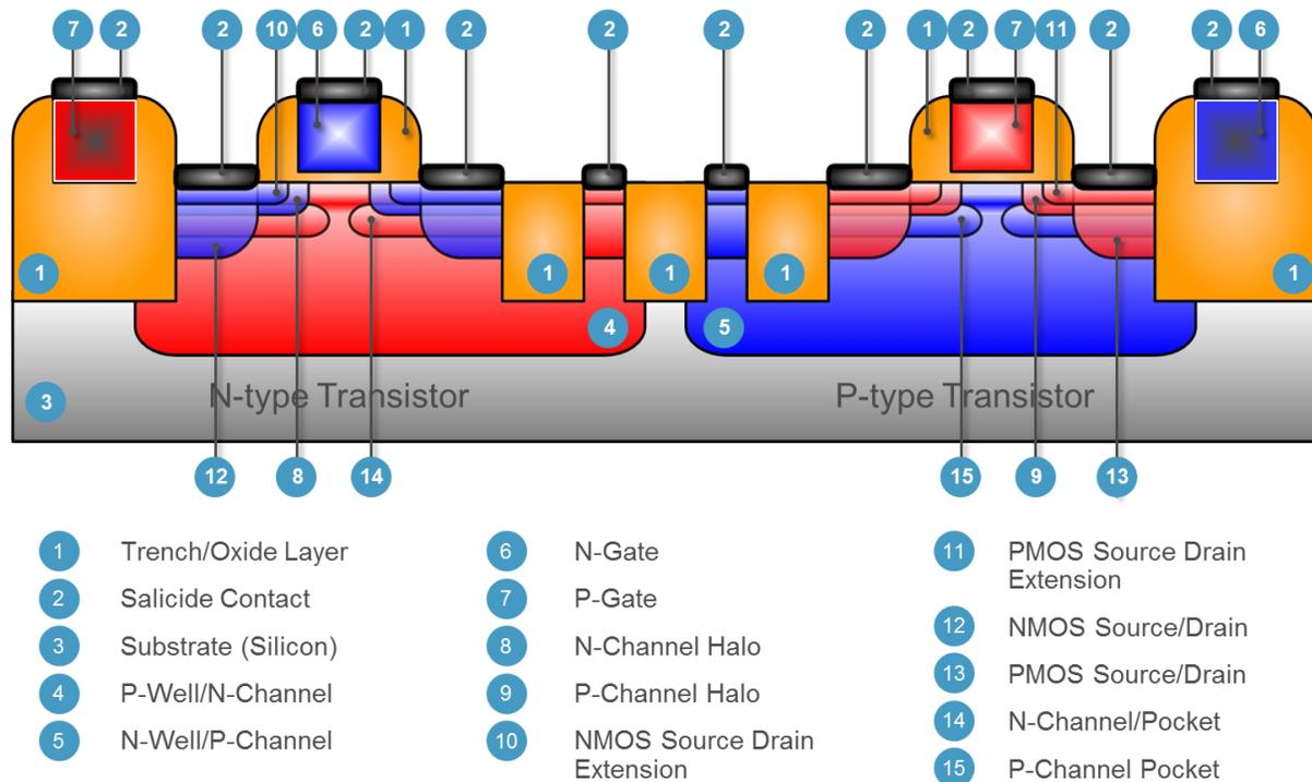
**Figure 1.** Fabricating today's complex chips can involve several dozen implant processes to promote or control current flow.
