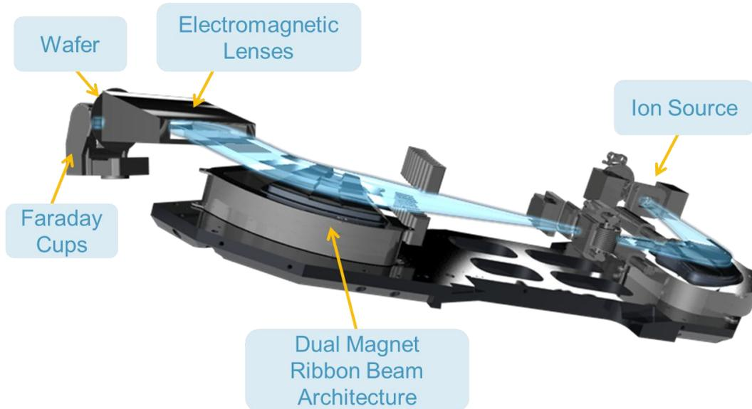
**Figure 2.** Ion implant systems use electromagnets and electrostatic lenses to filter out and steer the dopant ions from the source to the wafer surface, measuring ion density and angle of incidence using Faraday cups.
