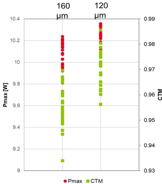
**Figure 3:** Pmax and CTM ratio plots of standard SHJ cells (160  $\mu\text{m}$ ) based shingle strings vs thinner-wafer cells (120  $\mu\text{m}$ ).
