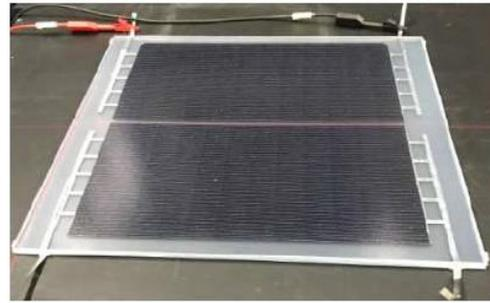
**Figure 2:** Test-module manufactured at CEA-INES, consisting in two independent strings of 12 cell stripes in series.
