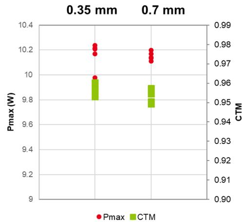
**Figure 4:** Power output and CTM ratio plots of back-side 0.35 mm vs 0.7 mm pitch cells configurations.
