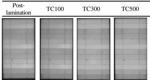
**Figure 6:** EL images of one 12-cells shingle string after the lamination process, after 100, 300 and 500 thermal cycles.
