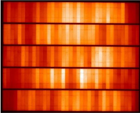
**Figure 8:** Post-lamination EL image of the half-module, with 5 strings of 37 cell in series each bussed in parallel.
