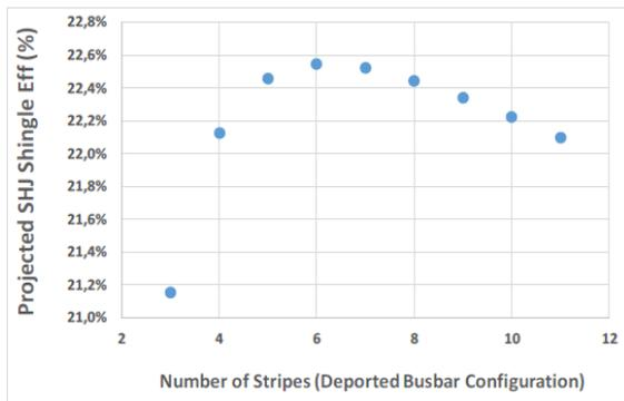
**Figure 1:** Calculated impact on efficiency of the number of SHJ shingle stripes considered for a given mother cell and usual low-temperature paste resistivity.
