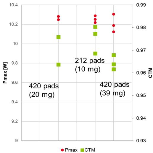
**Figure 5:** Power output and CTM ratio plots of different ECA quantities and metallic pad configurations.
