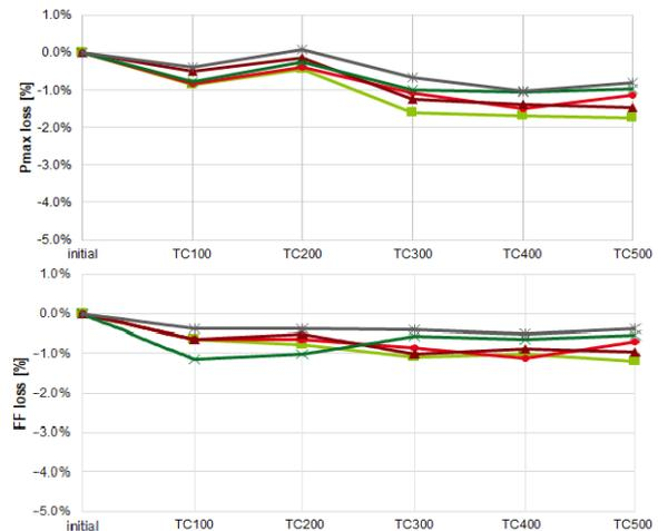
**Figure 7:** Power and FF losses evolution of the minimodules from the initial state to after 500 thermal cycles.
