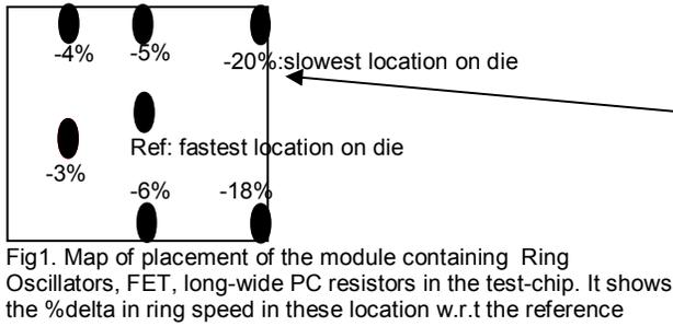
Fig1. Map of placement of the module containing Ring Oscillators, FET, long-wide PC resistors in the test-chip. It shows the %delta in ring speed in these location w.r.t the reference
