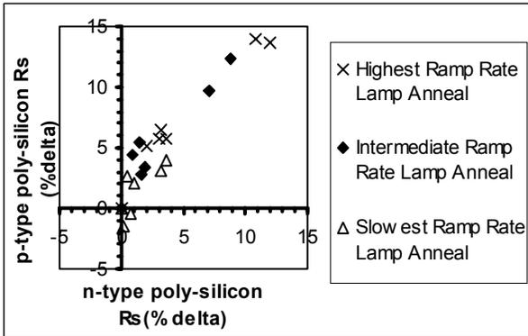
Fig.3 Large delta in unsolicited Poly sheet resistance noted at different locations in the die. Correlation between N and P Sheet resistance indicates *within-die* thermal absorption difference
