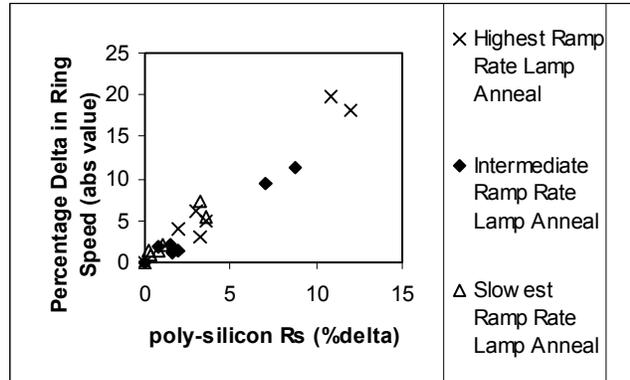
Fig4. Percentage delta in ring speed vs delta in unsolicited long-wide poly sheet resistance at different location in die indicating correlation between delta in *within die* thermal absorption and ring speed
