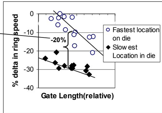
Fig2. All data from same wafer: Gate Length vs %Delta Ring Speed(delta to fastest ring on wafer) indicating that the large difference in ring speed in different location of the die for the same Gate length
