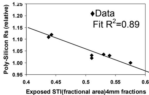
Fig8. unsolicited poly sheet Rs vs exposed STI density of the chip indicating strong dependence of thermal absorption on pattern density
