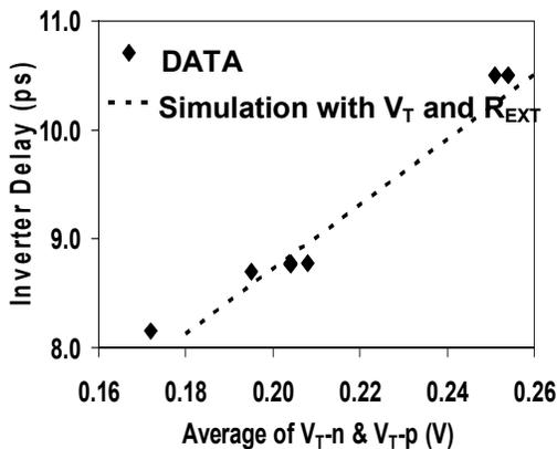
Fig7, Hardware vs Model correlation with model override for Rext and Vt for FETs indicating delta in ring speed is primarily coming from thermal absorption induced difference in Vt and Rext in the FETs.
