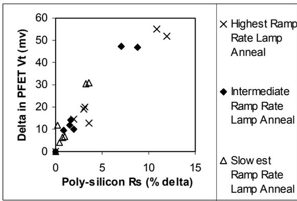
Fig5. *Within die* Percent delta in unsolicited Poly resistance vs *Within die* Delta Vt for PFET (abs. value) indicating Vt difference due to thermal absorption.
