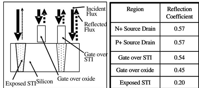
Fig. 1. Schematic and table of different reflection co-efficient of different exposed stacks in the absence of scattering effects [5].
