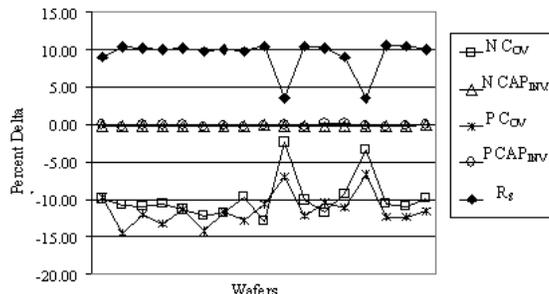
Fig. 7. Intra-die variation of different MOSFET parameters on an experimental lot, where two of the wafers were processed with a spike anneal with a lower ramp rate.
