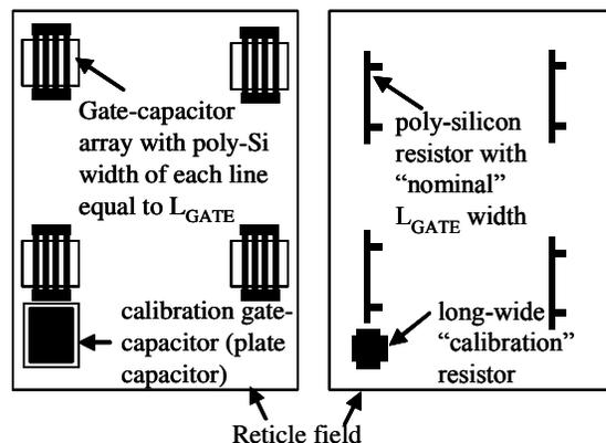
Fig. 5. “Resistive” and “capacitive” method of measuring  $L_{GATE}$
