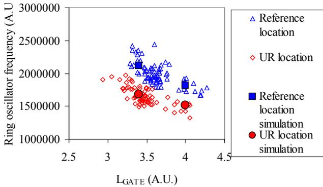
Fig. 9. Measured data and simulation: ring oscillator frequency vs  $L_{GATE}$ . The  $L_{GATE}$  measurement was done using the capacitive technique. The good agreement between simulation and measured data indicates consistency and accuracy in the measurement data of  $L_{GATE}$ .
