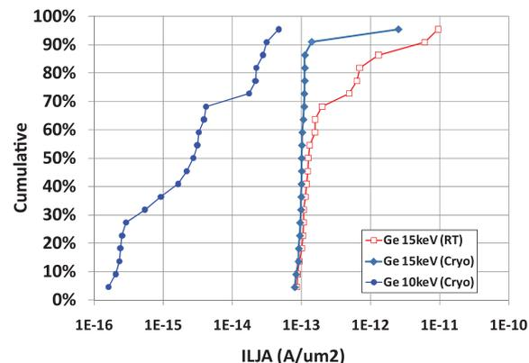
**Figure 3.** Junction leakage comparison for RT and cryo implants for Ge at either 15 or 10 keV. Ge 10 keV cryo-implants showed  $\sim 2$  orders leakage mean value reduction relative to Ge 15 keV RT implant conditions.
