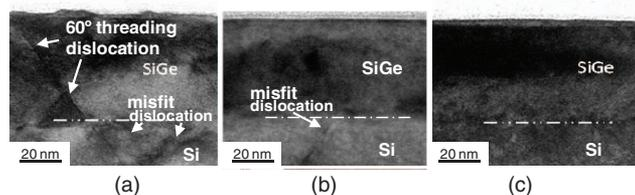
**Figure 2.** XTEM after spike/msec anneal for PSD implants at (a) Ge 15 keV at RT, (b) Ge 15 keV at cryo temperature, (c) Ge 10 keV at cryo temperature ( $-100^\circ\text{C}$ ).
