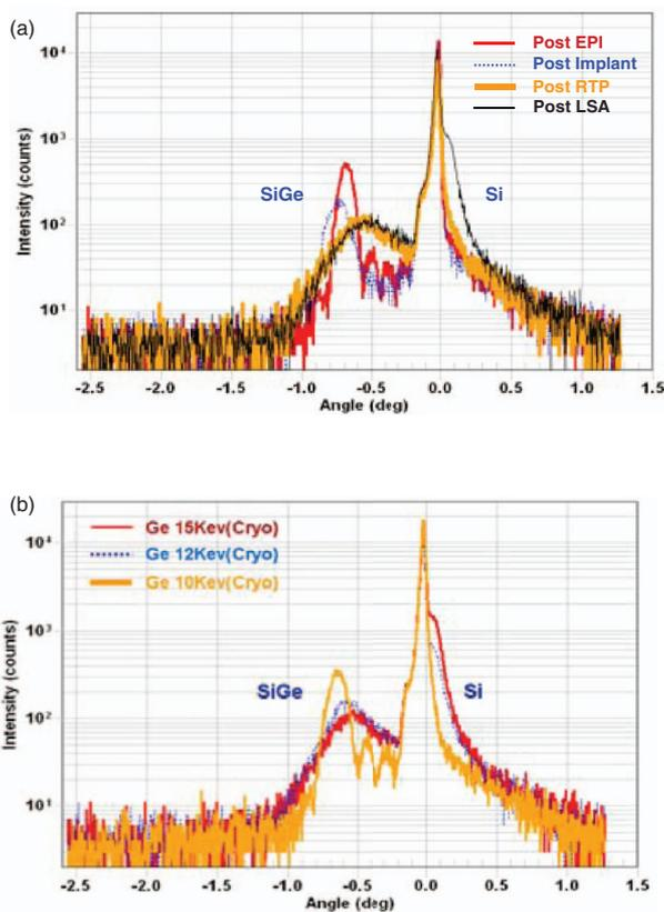
**Figure 1.** (a) HRXRD rocking curves for eSiGe/Si strain relaxation collected after SiGe EPI deposition, SD implant (Ge 15 keV,  $5 \times 10^{14}$  atoms/cm<sup>2</sup>), sRTP, and msec anneal, respectively. (b) HRXRD rocking curves for Ge energy response (10, 12, and 15 keV) after anneal (sRTP/msec) coupled with cryo temperature ( $-100^\circ\text{C}$ ).
