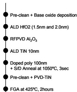
Figure 1 Process Flow
