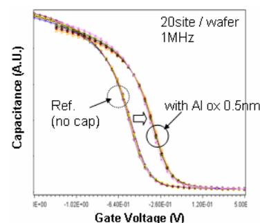
Figure 2 20 site C-V curves with and without RFPVD Al oxide cap layer on 2.0nm  $\text{HfO}_2$ . C-V curves show uniform  $V_{FB}$  shift by  $\text{AlO}_x$  cap layer across the wafer.
