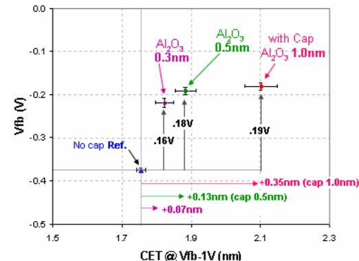
Figure 4 CET- $V_{FB}$  plot of samples with various Al oxide cap thickness; 0, 0.3, 0.5 and 1.0nm on 2.0nm  $\text{HfO}_2$ . 0.5nm cap shows equivalent  $V_{FB}$  shift,  $\sim 0.2\text{V}$ , to 1.0nm cap with minimal CET increase,  $\sim 0.1\text{nm}$ .
