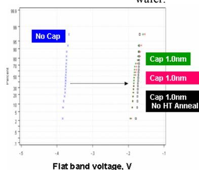
Figure 3 Probability plots of  $V_{FB}$  with and without 1.0nm Al oxide cap and HT anneal.
