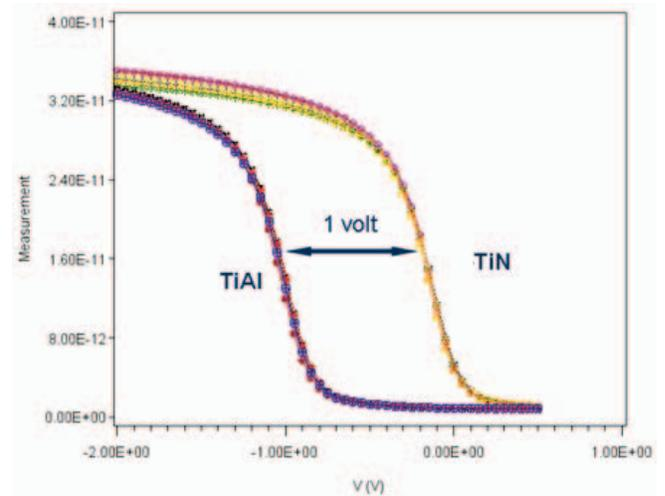
Figure-8: C-V measurements of TiN (PMOS) and TiAl (NMOS) deposited in replacement gate scheme showing 1 volt separation. Multiple curves per condition represent within wafer uniformity of the stack films.
