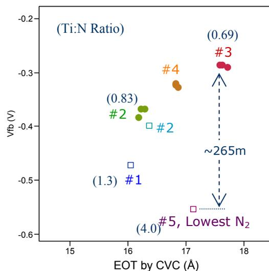
Figure-3: Impact of Ti:N<sub>2</sub> stoichiometry on flatband voltage of HfO<sub>2</sub>/TiN stack layers in gate first integration
