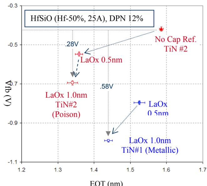
Figure-4: Flat-band voltage ( $V_{fb}$ )-EOT of  $LaO_x/TiN$  stack in gate first scheme. TiN#2 is poison mode TiN.
