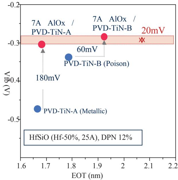
Figure-5: Flat-band voltage ( $V_{fb}$ )-EOT of  $AlO_x/TiN$  stack in gate first scheme.
