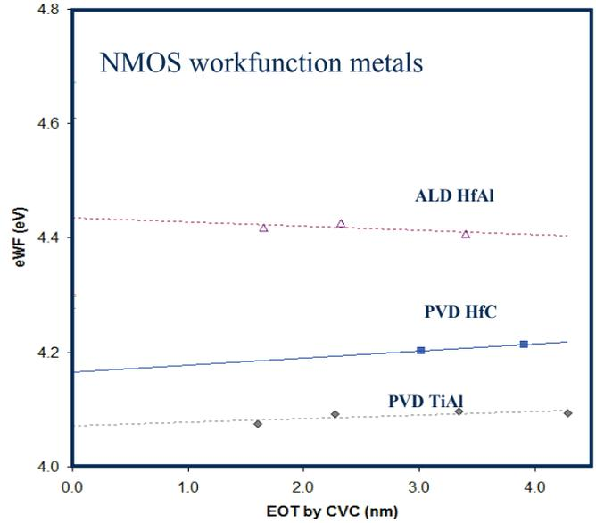
Figure-7: Workfunction screening of NMOS metals in replacement gate (high-k first, metal gate last) integration flow
