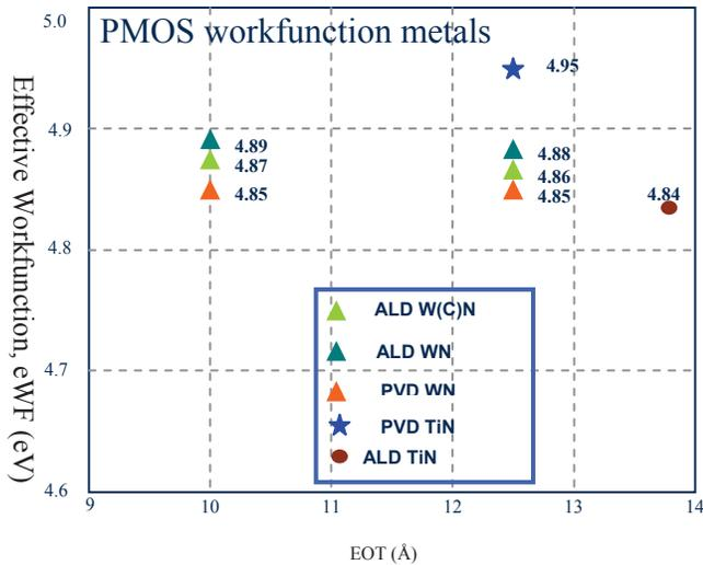
Figure-6: Workfunction screening of PMOS metals in replacement gate (high-k first, metal gate last) integration flow
