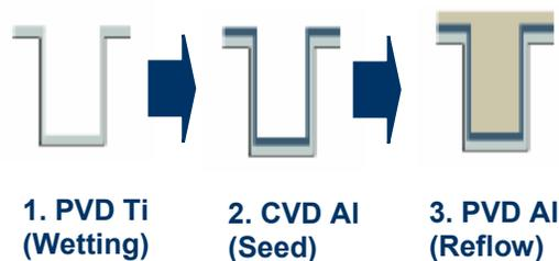
Figure-2: Process flow of Al gap fill containing Ti wetting layer, Al seed and reflow layers.
