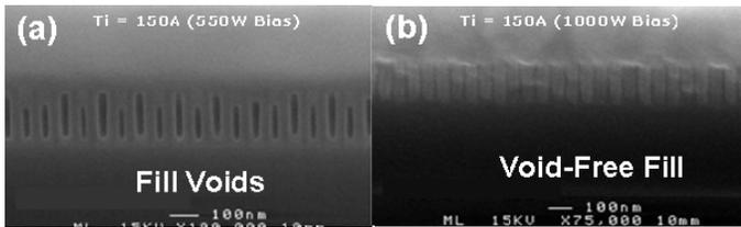
Figure-9: Impact of substrate bias of PVD Ti wetting layer on gap fill
