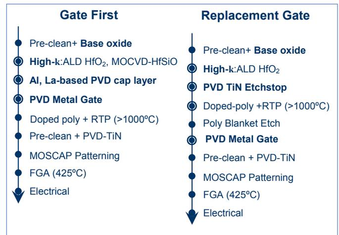
Figure-1: MOS-fabrication flow used for GF and RG flows. Two integration flows were used in RG – high-k first/metal last and both high-k last/metal last.
