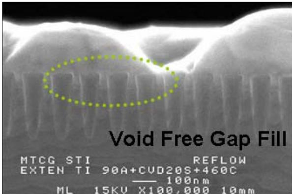
Figure-10: Void-free Al gap fill achieved by preferential liner treatment of PVD Ti wetting layer in  $N_2$  plasma
