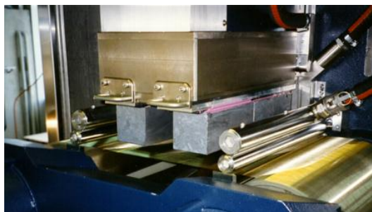
Figure 2: Silicon blocks are passed through the web of cutting wires.
